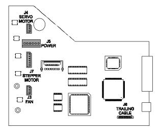
Figure 3-4. MPCB Connection Locations.
